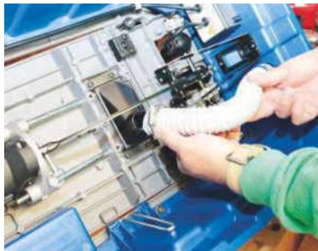
You have to connect the supplied link hose if you want to use an extractor
